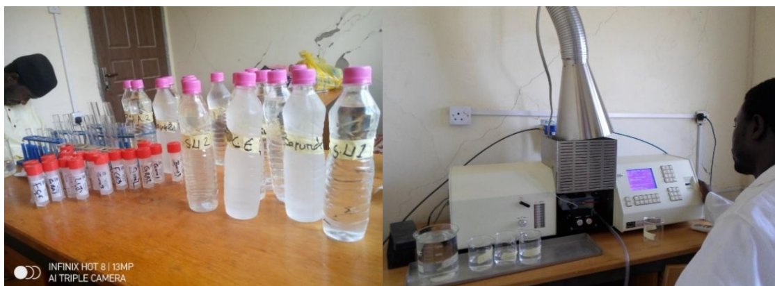
Plate 1: Collected labelled Water Sample and Atomic Absorption Spectrophotometer (AAS) used Source: Author, 2024
